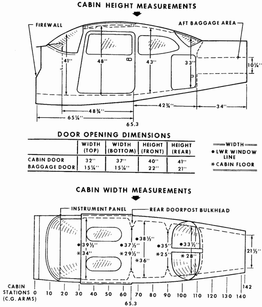
Figure 6-4. Internal Cabin Dimensions
