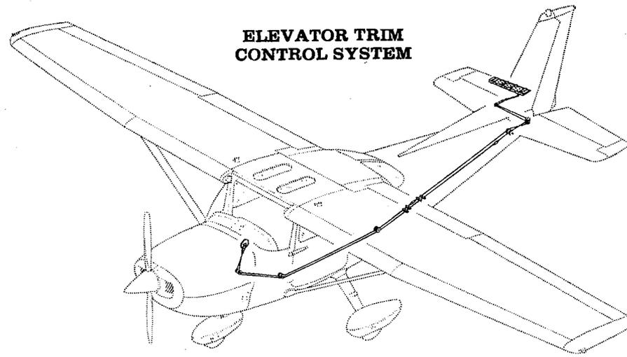
Figure 7-1. Flight Control and Trim Systems (Sheet 2 of 2)
